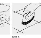
Leave the wax for 20 minutes and then buff to a shine using a stiff buffing brush for small spaces or a mechanical buffing machine and brush (available from hire shops) until the wax shines.\*
