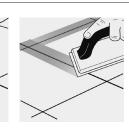
**STEP 3.** Leave wax to cure for 1 hour and then grout the joints.
