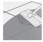
Scrub surfaces and grout joints using a white emulsifying pad to release the dirt and grime.
