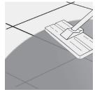
Working in manageable areas at a time when applying the solution to the surface. Leave for 15 minutes.
